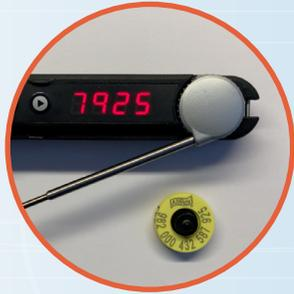
If during the original 12 second window the RFID number was not found, the operator can press the **Start** button twice to cycle back to obtain the ID number.
