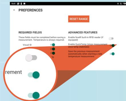
If feveR is **not** set on the **QT** setting the device will **continuously** monitor the temperature until the operator is satisfied and pushes the **Start** button to stop the reading.
